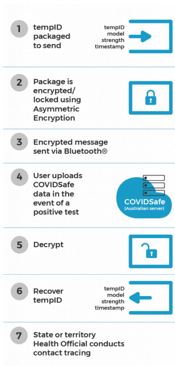
Figure 1: data sent in the digital handshake is now encrypted, so only the COVIDSafe server can read it
